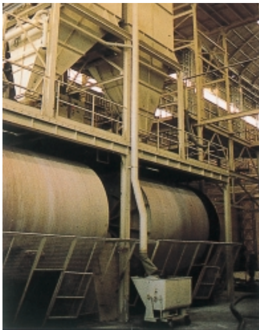
Mills for wet grinding of tile body raw material.
